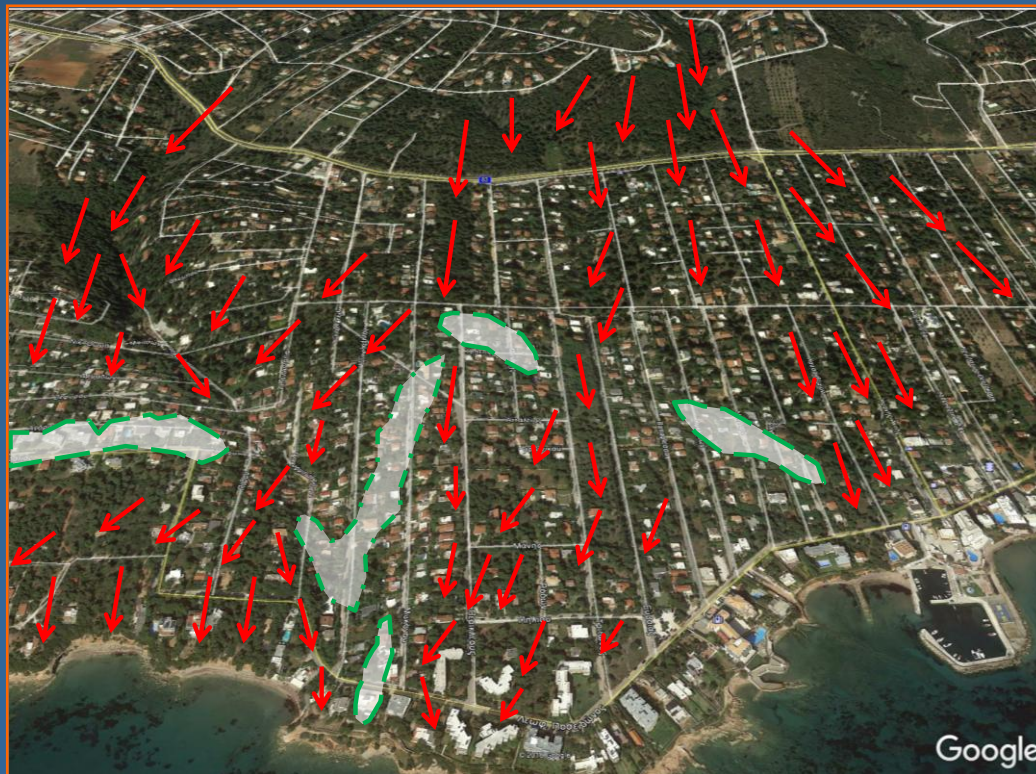
Vectors of wildfire uninterrupted spread mapped with the aid of UAV footage from Neos Voutzas to Mati.
