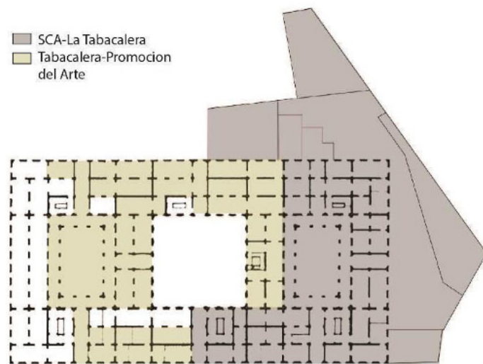
Fig 30 Distribution of new functions in the former tobacco factory (Source: Dora Chatzi Rodopoulou Archive)
